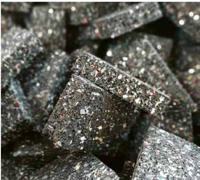
Isopads made of 95% discarded tyre granulate
